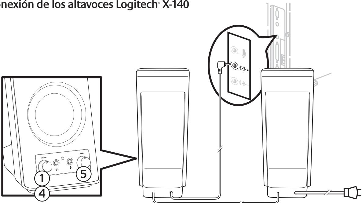
Connect your Logitech® speakers to your soundcard, or external audio source, following the diagram above. The speaker with the volume control is the right channel. Note: If your soundcard has both a line level output and a speaker output, use the line level output.
