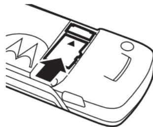
down, and slide the top of the memory card under the metal band.
