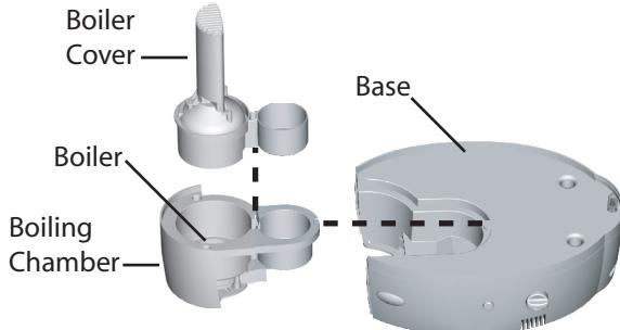
4. Place the Boiling Chamber into an empty sink and carefully lift the Boiling Chamber Cover by pressing the Chamber Cover Release Tab. This will expose the Heater. Drain all water and rinse with cool, clean water. Use a soft brush or sponge to clean the Boiling Chamber and the Boiling Chamber Cover.
