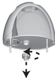
5. Replace the Tank Cap by screwing it clockwise onto the Water Tank.
