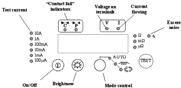
Press the On/Off switch to turn DLRO 10 on. All lamps will light, V and I lamps will flash, the software version will be displayed and the  $\Omega$  lamp will light. If the test leads have not been connected to the test sample the 'C' and 'P' lamps will also light. Press the On/Off button again to turn the instrument off. If the instrument is not used for 5 minutes it will be turned off automatically.
