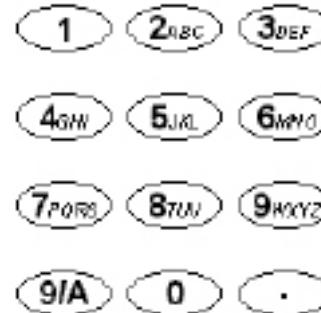
Pressing the blue key marked 9/A changes the function of the keyboard between alpha and numeric modes.
