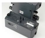
The DLRO10 and DLRO10X may be also powered from an optional mains / line power supply unit the DLRO10LPU. This unit is simply fitted to the instrument in place of the standard battery pack.
