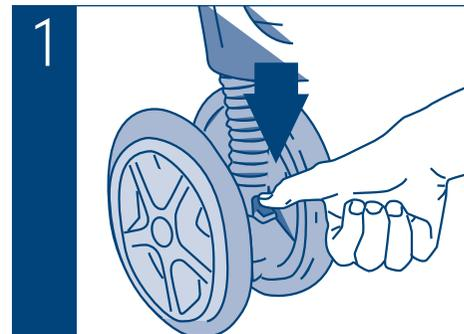
The swivel wheel should be locked for use on uneven surfaces such as gravel, grass or stones. To lock the swivel, press down on the lever as shown. Lift up to unlock.
