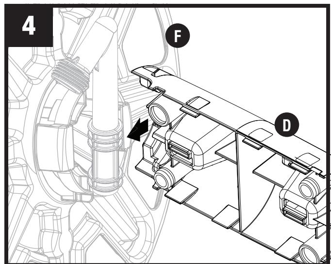
Align tabs on crossbrace (D) to reel side (F). Snap left crossbrace into left reel side.
