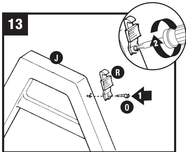
Secure catch (O) with screw (R) to rear upright of a side frame (J). Repeat for other side frame (M).
