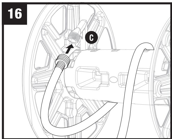
To connect garden hose, thread end of garden hose onto out-tube (C) as shown.
