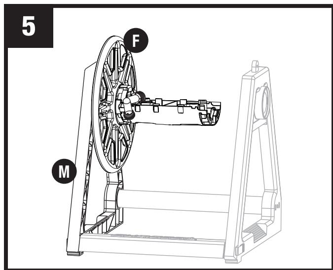
Place left reel side (F) next to the left side frame (M) so that the cylinder goes inside the side frame.
