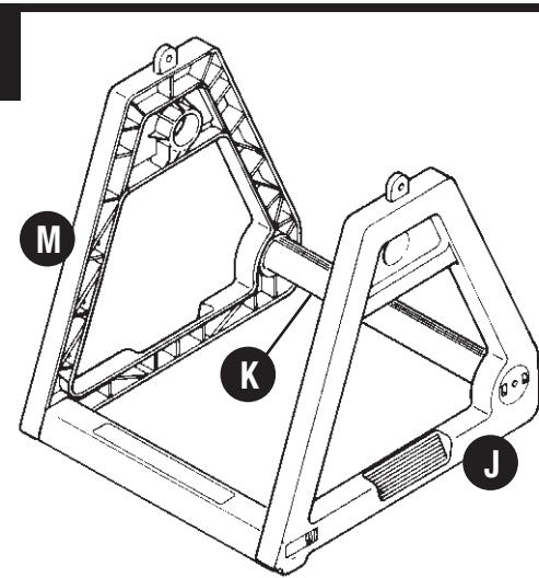
Snap frame bar (L) into right side frame (K). Repeat for left side frame (M).
