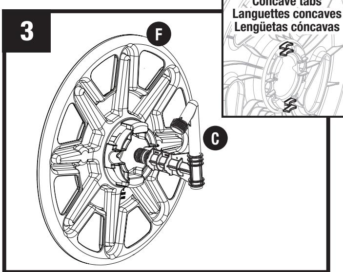
Put out-tube (C) into left reel side (F) making sure that it rests against two concave tabs on the inside of the reel.
