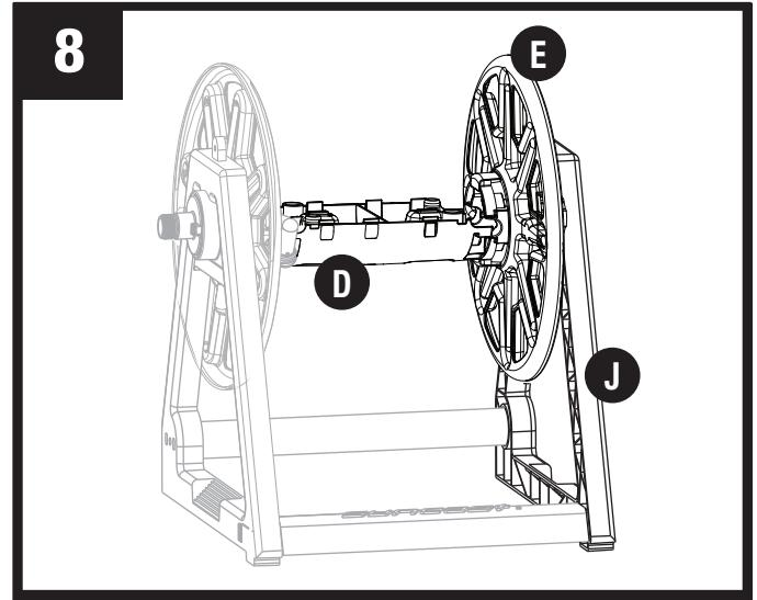
Place right reel side (E) next to the right side frame (J) so that the cylinder goes inside the side frame. Snap crossbrace (D) into right reel side (J).
