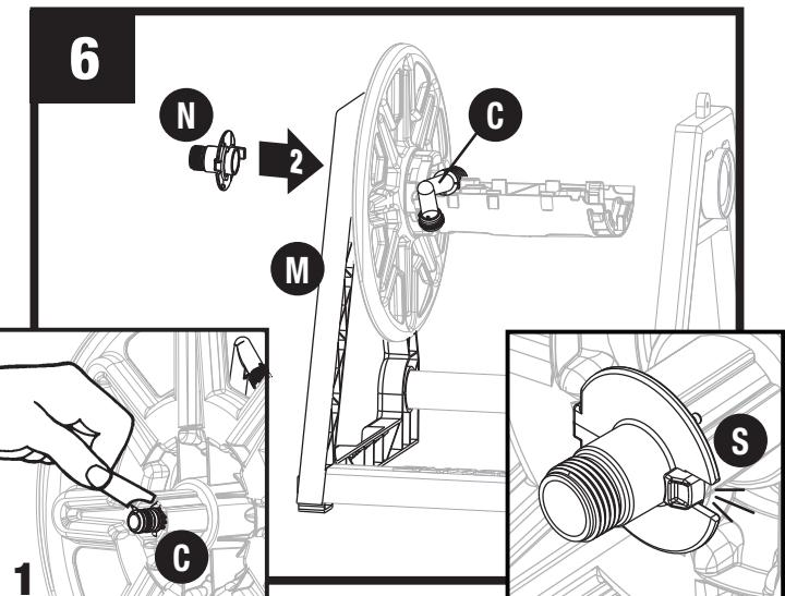
Open lubricant tube (included) and smear contents on o-rings of out-tube (C). Hold onto out-tube (C) while fitting supply tube (N) into side frame (M).
