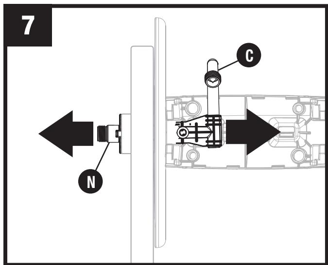
**CRITICAL** – Make sure tubes (N/C) are fully engaged by pulling each tube outward. If not fully engaged, repeat Step 6.
