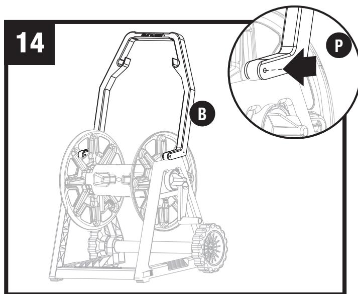
Place handle (B) on frame as shown. Tap hinge pins (P) through mating holes to secure handle.
