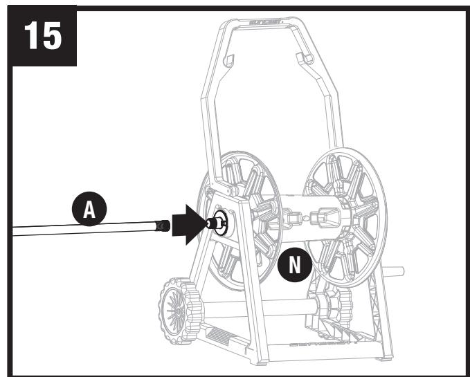
To connect leader hose (A), thread end of leader hose into supply tube (N). Thread end of leader hose onto faucet.
