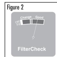
When the needle is in the CHANGE section, this means the proper amount of moisture is not getting into your air due to the excessive minerals and sediment that have become trapped on your filters. At this point, you should replace your filter. It is important to change your filter as indicated to obtain stated performance level.
