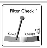
When the needle is in the red (CHANGE) section, this means the proper amount of moisture is not getting into your air due to the excessive minerals and sediment that have become trapped on your filter. At this point, you should replace your filter. It is important to change your filter as indicated to obtain stated performance level.
