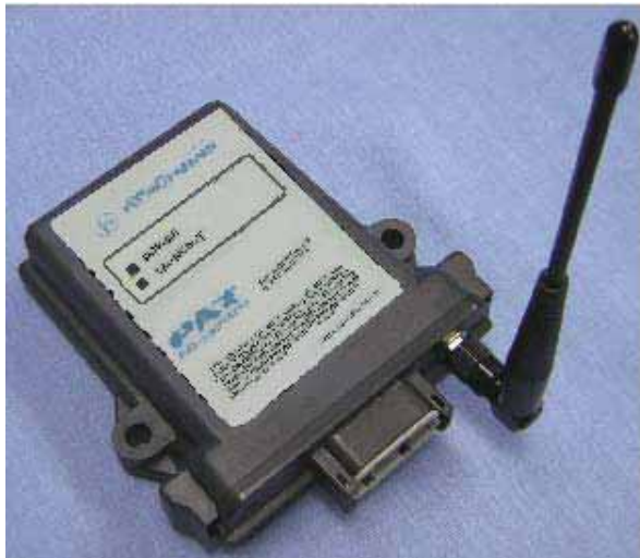
031-300-060-596 TRS 05 REPEATER 031-300-050-688 ANTENNA, 918 MHz RCL 90°
