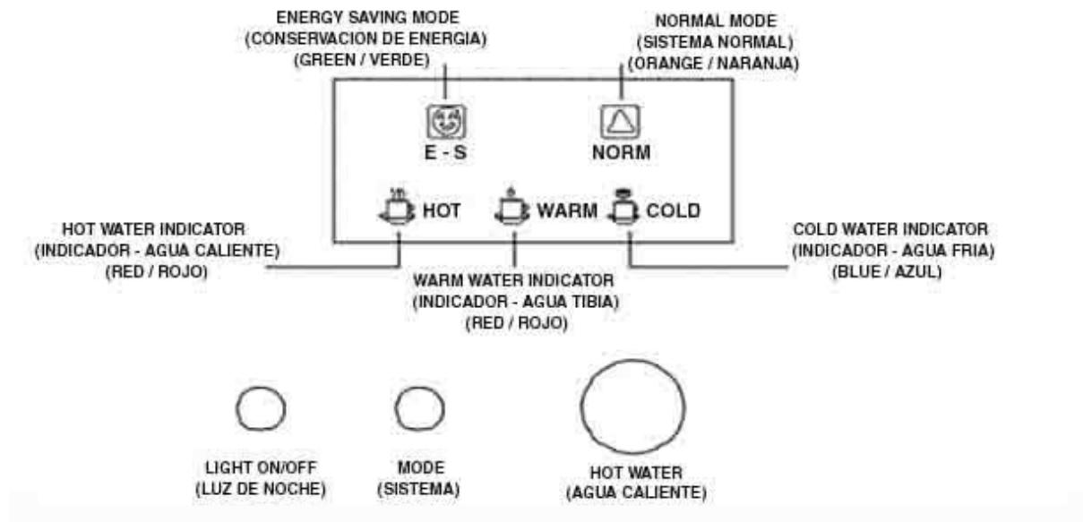
For operation of unit, please fill water and make sure water settles inside the water tank, and then switch on both hot and cold switches at back of unit.
