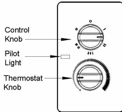
Fig. 4 - Controls & Control Panel Layout
