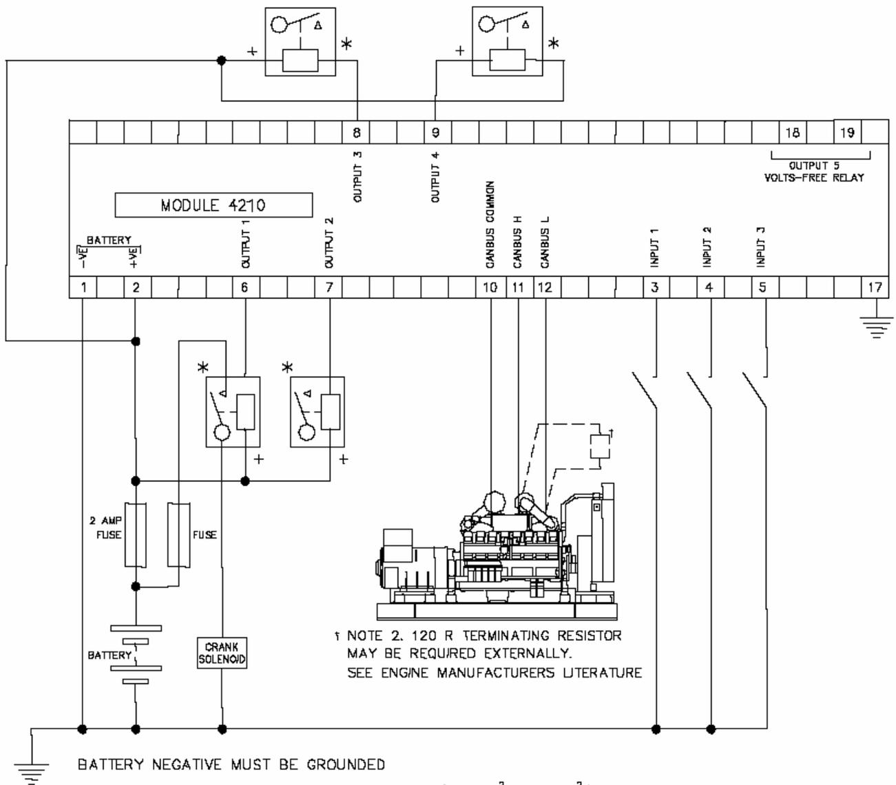
TERMINALS SUITABLE FOR 22-16 AWG (0.6mm<sup>2</sup> - 1.3mm<sup>2</sup>) FIELD WIRING
