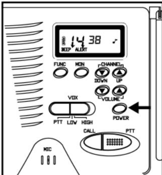
**Adjusting the Speaker Volume** - With the radio on, press the VOLUME UP ( $\blacktriangle$ ) button to increase volume; press the VOLUME DOWN ( $\blacktriangledown$ ) button to decrease volume. The volume indicator icon (number 1 - 8) will change according to your setting. Hold the VOLUME UP ( $\blacktriangle$ ) or DOWN ( $\blacktriangledown$ ) button to scroll through settings. A double beep will sound when the volume reaches the highest (8) and lowest (1) settings.
