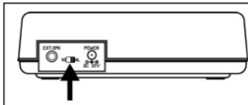
The **NI / AL Switch** is located on the back of cabinet. Select switch position by battery type.
