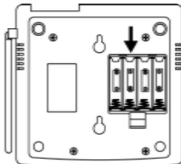
The **Battery Door** is located on the base of cabinet. Press tab down to open the door; load batteries following the polarity diagram embossed in cabinet.
