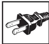
THIS APPLIANCE HAS A POLARIZED PLUG (one blade is wider than the other). To reduce the risk of electric shock, this plug is intended to fit in a polarized outlet only one way. If the plug does not fit fully in the outlet, reverse
