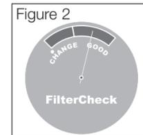
section, this means the proper amount of moisture is not getting into your air due to the excessive minerals and sediment that have become trapped on your filters. At this point, you should replace your filters. It is important to change your filters as indicated to obtain stated performance level.
