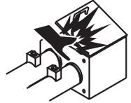
THE LUBRICATION BOX CONTAINS MOVING PARTS. DO NOT PUT HANDS OR OTHER BODY PARTS IN THE LUBRICATION BOX WHILE THE PUMP AND ENGINE ARE RUNNING.
