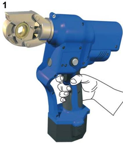
The **crimping operation** is carried out automatically on pressing the black push button on the handle.
