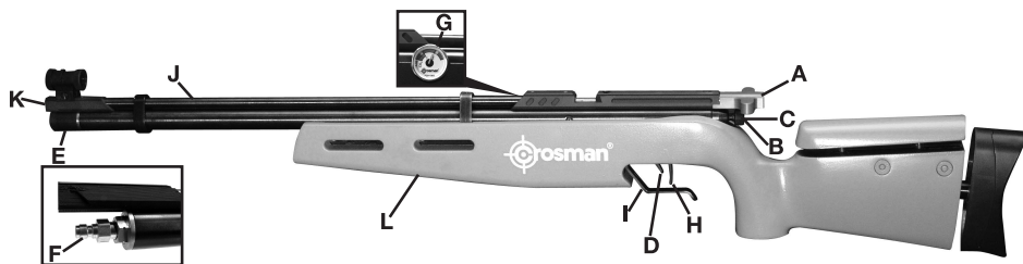
A. Bolt B. Hammer spring adjustment knob C. Hammer/ Striker travel adjustment (internal- accessed through Hammer spring adjustment knob) D. Safety E. Protective cap for fill nipple F. Fill nipple G. Pressure gauge H. Trigger I. Trigger guard J. Barrel K. Muzzle L. Stock
