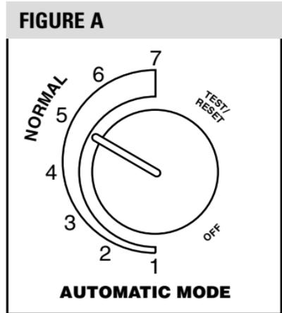
Your Aprilaire Automatic Humidifier, is a high precision system that will accurately maintain the relative humidity in your home. For every 1° change in outdoor temperature, the control will automatically adjust the indoor relative humidity (RH) by 1/2%. If you would like to determine the RH in your home, follow these steps:
