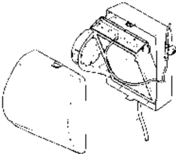
1. Note Humidifier Control setting and turn dial to the "OFF" position.
