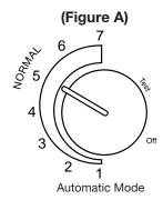
Your Aprilaire Automatic Humidifier, is a high precision system that will accurately maintain the relative humidity in your home. For every 1° change in outdoor temperature, the control will automatically adjust the indoor relative humidity (RH) by ½%. If you would like to determine the RH in your home, follow these steps:
