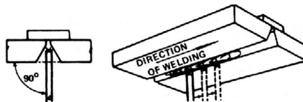
Figure 3.40 Overhead Butt Weld - Root Pass
