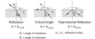
In the MA871, light from an LED passes through a prism in contact with the sample. An image sensor determines the critical angle at which the light is no longer refracted through the sample. The MA871 automatically applies temperature compensation to the measurement and converts the refractive index of the sample to sucrose concentration in units of percent (by weight) Brix.
