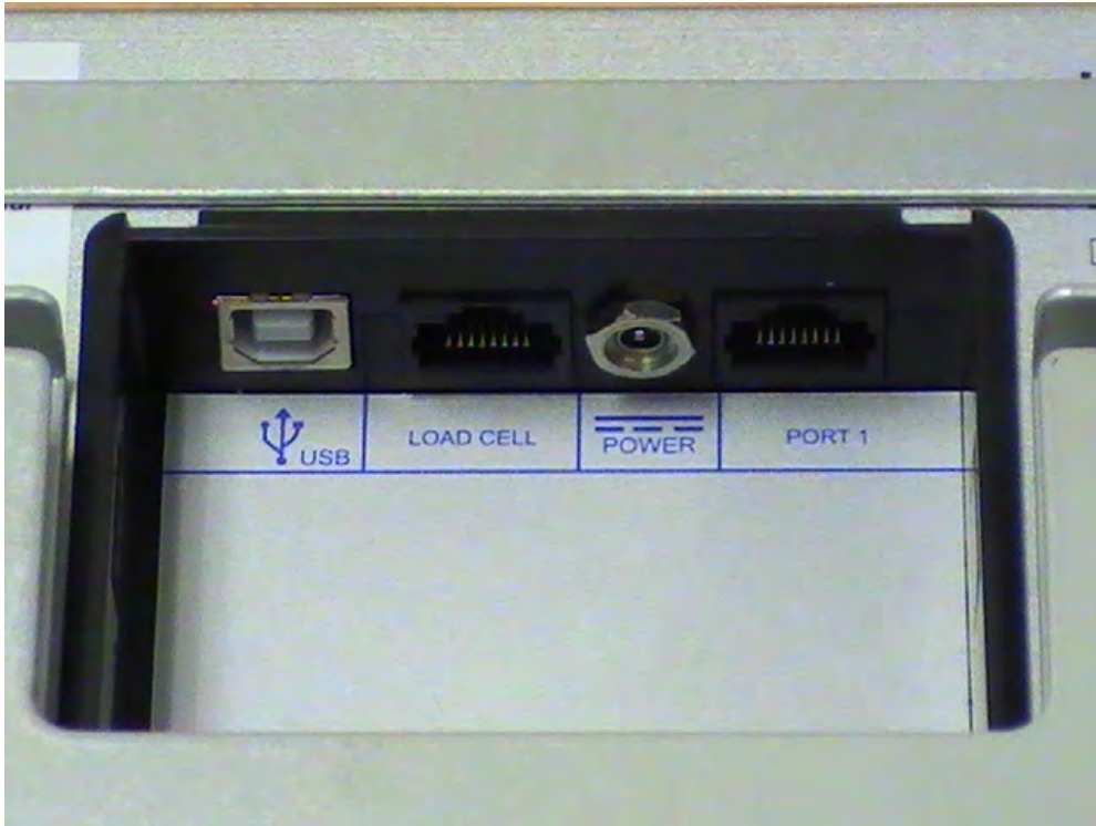
Rear of Display Head on 2500KL and 2600KL
