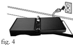
1. Place the Grill & Panini Press on a dry, stable surface away from an open flame or hot burners. Open the upper housing by the handle to an upright position and then press the hinge release button on the side of the hinge to move the upper plate to a flat position (see Fig.1). This appliance requires 1400 watts and should be the only appliance operating on the circuit. Plug the unit into a 120 volt 60 Hz AC outlet only.
