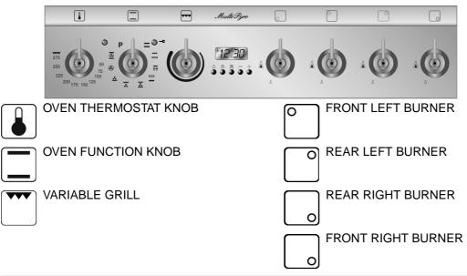
Before using the oven make sure that the symbol  $\stackrel{JJJJ}{\amalg}$ ; appears on the display. See paragraph "11. ELECTRONIC PROGRAMMER".
