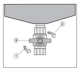
Make sure that the underside of the grill is left accessible for draining the water. Wait until the water has cooled down before draining to prevent scalds.
