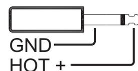
Fig4. Jack Unbal Input / Output Pin-out
