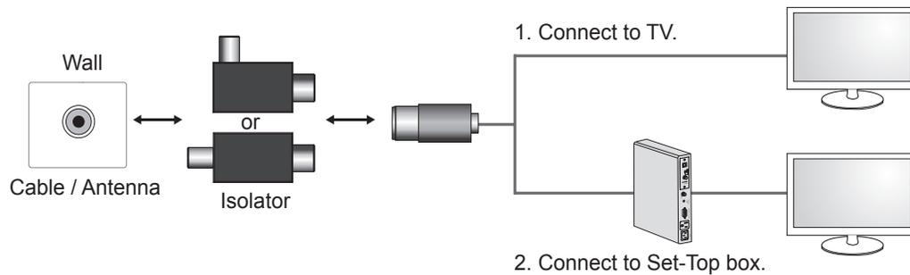
Connect one end of the isolator to cable/antenna jack and the other to TV set or set-top box.
