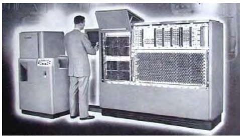
The UNIVAC 120 was a 1953 release of a modified Remington Rand Model 409 computer.
