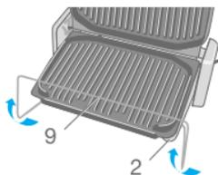
Swing the support wire (9) forward to lift up the lower section (2) of the appliance: the grill plate is then in a horizontal position.
