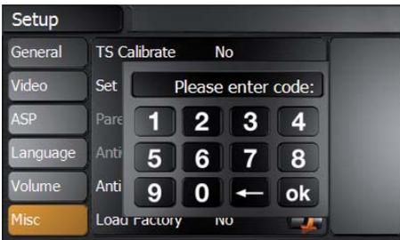
2. Touch the anti-theft code icon and use the keypad, which appears on the screen, to enter the four-digit anti-theft code and confirm your input by entering the same code a second time.
