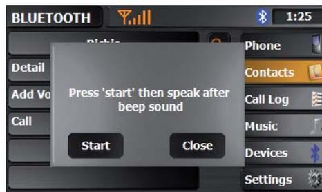
3. To start a call using a voice tag: Touch the [📞]-icon two times and wait with the speech input until an acoustic beep signal is audible. If the speech input meets the recorded voice tag, the unit starts to dial the phone number of the entry.
