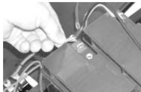
FIGURA 12. DISTACCO DEI CAVI BATTERIE
