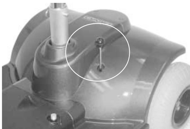
FIGURA 7. LEVA SBLOCCO RUOTE MANUALE
