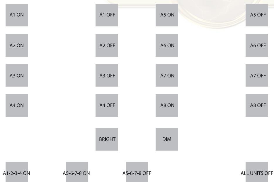
If you press on the first button, then address A1 ON will be sent. The appliances and/or lights that are at the address (A1) will, therefore, go ON. And so on.
