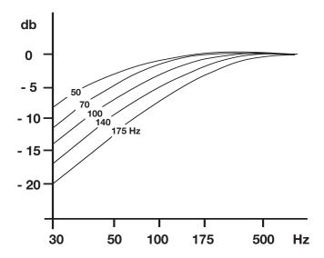
You will need to use your ears to determine the best settings for these filters. The frequency markings shown next to each control knob may give you some guidelines. 50Hz (or above) might be used as a setting for music production. 80Hz is the proposed setting for Dolby Digital playback, while 100Hz is the proposed setting for THX.
