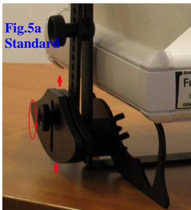
**Balance the rotating arm** (with the camera mounted)
