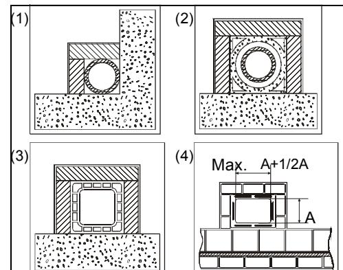
(1) AISI 316 steel flue with double chamber insulated with material resistant to  $400^\circ\text{C}$ . **Efficiency 100% excellent.**
