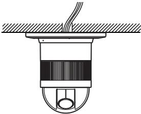
1. Mark the mounting holes on the ceiling, using the removed camera mounting base as a template.
