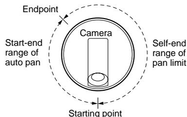
**Note:** When ON is selected for PAN LIMIT, manual pan moves the camera away from the other side (PAN LIMIT) of the start-end range.
