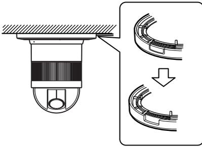
**Note:** Remove sharp edges to protect the cables.
