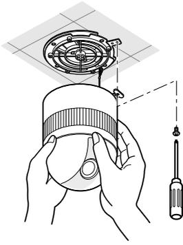
5. Tighten the fixing screw M3 (provided).
