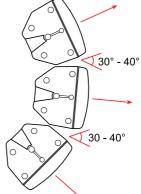
Correct positioning of the cabinets: an angle within 30°/40° minimizes horns interac-30° - 40° tion and gives a linear frequency response.
