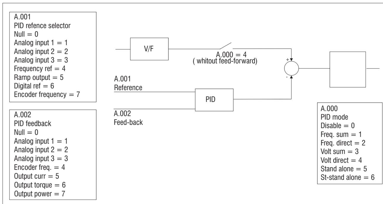
Figura 1.1-3: PID Mode as Voltage Sum or Direct
