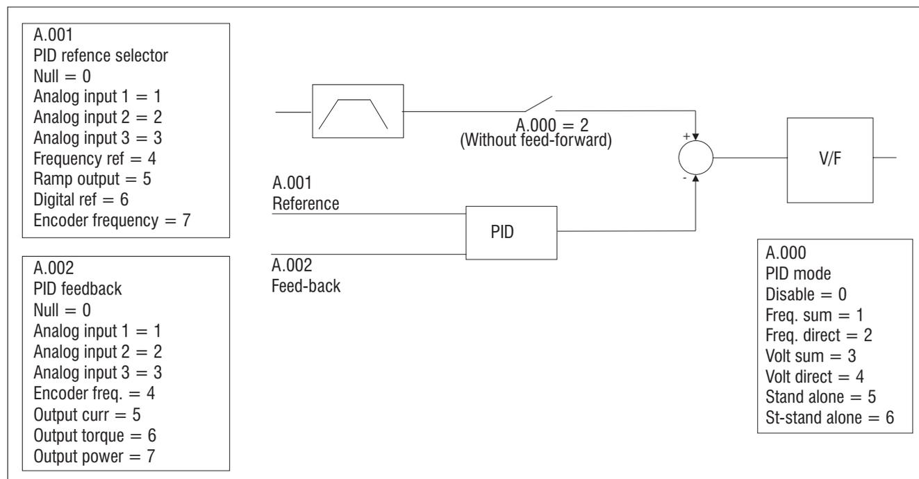
Figura 1.1-2: PID Mode as Frequency Sum or Direct
