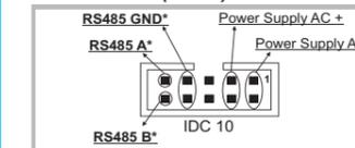
In the figure the meaning of the IDC10 connector pins is showed, in the case the user decides to provide the signals directly through it.
