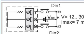
An external power supply from 12 to 30 Vdc can be connected to the input terminal. All the inputs are connected in shared connection to terminal 8 (GND). The current that flows through a closed input is approx. 7mA.
