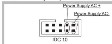
In the figure the meaning of the IDC10 connector pins is showed, in the case the user decides to provide the signals directly through it.
