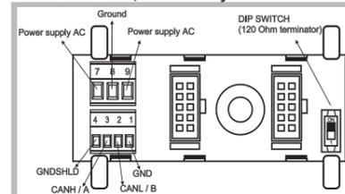
In case of Z-PC-DINAL2-17,5 accessory use, the signals may be provided by terminal blocks. The figure shows the meaning of the terminals and the position of the DIP-switch (present on each DIN rail supports listed on Accessories) for network termination (not used in case of Modbus network). GNDSHLD: Shield to protect the connection cables (recommended).
