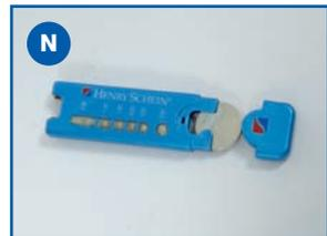
**NOTE:** When storing the **Digital Apex Locator** for an extended period of time without use, it is recommended to remove the battery from the device in order to lengthen the battery life.
