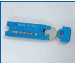
Replace with a fresh battery (type CR2450). Be sure to insert the battery into the drawer with the + sign facing upwards. Slide the drawer back into the battery housing with the + sign to the REAR of the device.
