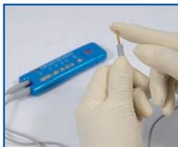
◀ Insert the mini file holder and lip hook into the sockets located at the end of the lead wires (either left or right).
