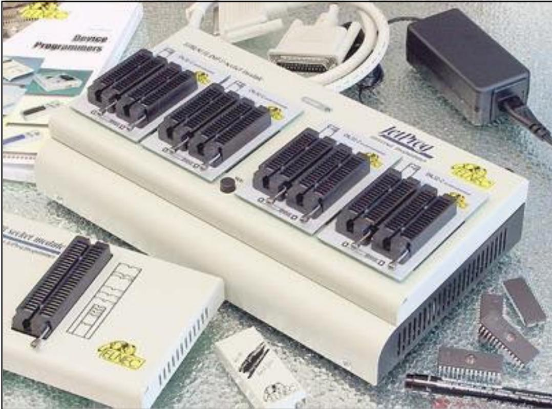
FIGURE 1: PHOTO OF JETPROG WITH EPROM/FLASH MODULE AND DIL32-2 SUBMODULES
