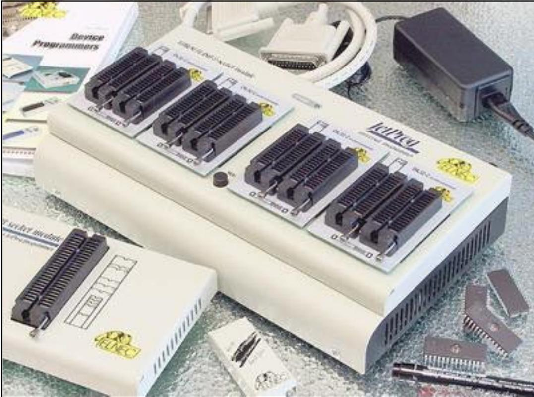
FIGURA 1: FOTO DEL JETPROG CON MODULO EPROM/FLASH E SOTTOMODULI DIL 32
