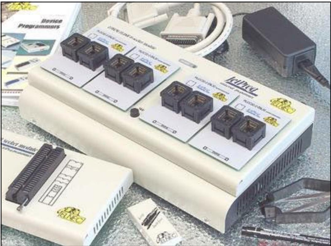
FIGURE 2: PHOTO OF JETPROG WITH EPROM/FLASH MODULE AND PLCC32-2 SUBMODULES
