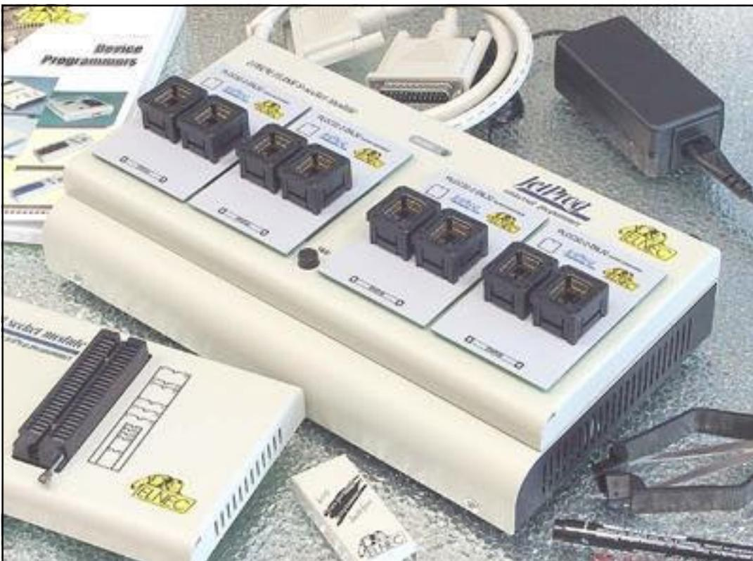
FIGURA 2: FOTO DEL JETPROG CON MODULO EPROM/FLASH E SOTTOMODULI PLCC 32
