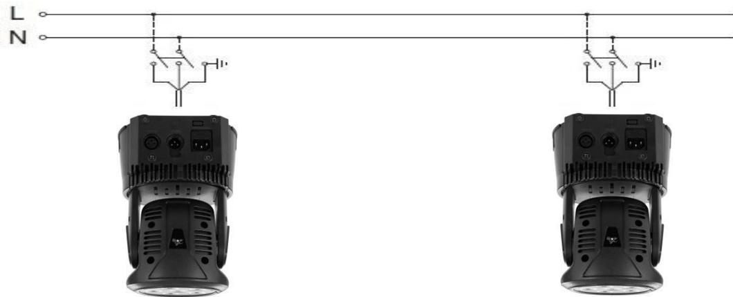
The device must be connected to a power supply system with a proper earth system. Moreover, it is recommended to protect power supply lines of the products from indirect contact and / or shorting to earth by using appropriately sized anti electrical shock switch. The electrical connection must be carried out by a qualified electrician. Ensure that the mains frequency and voltage correspond to those for which the device is designed, as shown in the electrical data label.
