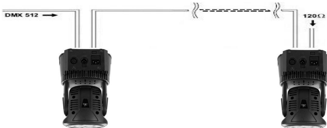
Use a cable conforming to specifications EIA RS-485: pole twisted, shielded, 120Ohm characteristic impedance and low capacity (PROEL DMXD – DMXD1).
