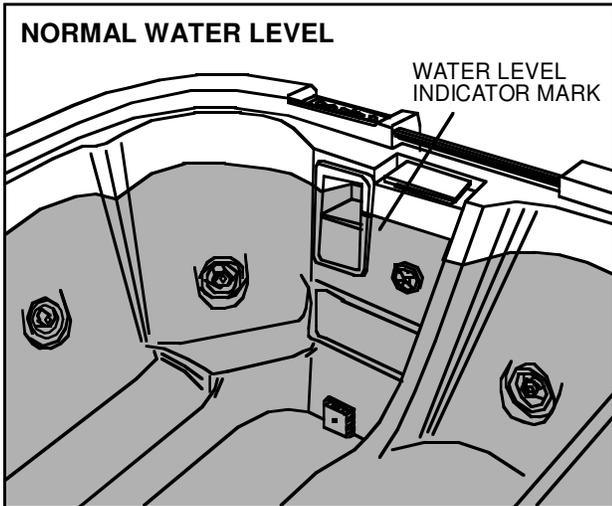
The suction strainers located in the foot well area should be checked at least once a week for collected debris, such as leaves, hair, etc., and cleaned as necessary. It may not be necessary to remove the strainer to clean it, but should you need to, remove the center screw with a Phillips type screwdriver and clean the strainer by flushing with water from a hose.
