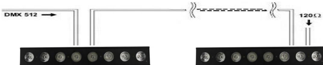
Use a cable conforming to specifications EIA RS-485: pole twisted, shielded, 120Ohm characteristic impedance and low capacity (PROEL DMXD – DMXD1).
