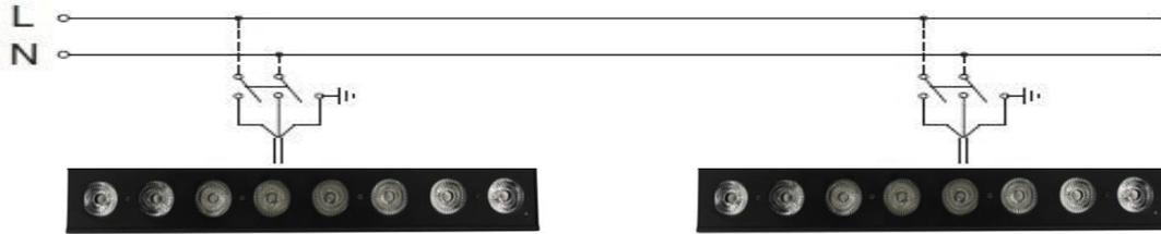
The device must be connected to a power supply system with a proper earth system. Moreover, it is recommended to protect power supply lines of the products from indirect contact and / or shorting to earth by using appropriately sized anti electrical shock switch. The electrical connection must be carried out by a qualified electrician. Ensure that the mains frequency and voltage correspond to those for which the device is designed, as shown in the electrical data label.
