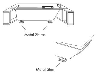
**Option For Sunken Installation:** Set the bath into the sunken installation. Make sure the unit is level and resting on all support feet. Insert the drain tailpiece into the trap. Apply a bead of silicone sealant under the rim of the unit.
