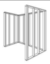
Sunken Installation: Refer to Roughing-In notes beginning on Page 1 for cut-out details. Make sure the whirlpool is supported by the supporting feet on the bottom of the whirlpool. Do not hang the whirlpool by the rim.
