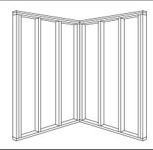
2. **Recess Installation:** The suggested stud construction is illustrated.
