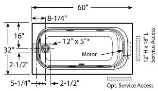
Product Shown: Luxura™ 5 Whirlpool Bath with 3 Tile Flange Left Hand Model: F941 \* Measurements inside unit represent cutout in floor to allow for drain/overflow. Minimum Service Access dimensions given.
