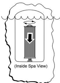
**H** Install filter cartridge back onto wall fitting by rotating the cartridge handle clockwise. **DO NOT OVERTIGHTEN!**
