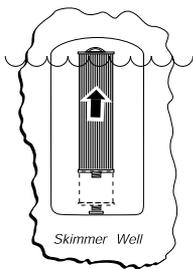
**E** Lift unthreaded filter cartridge from skimmer well.
