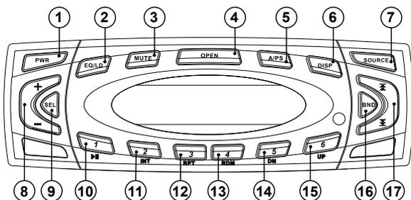
13. **Preset 4/RDM Button:** In tuner mode, any station can be stored as preset 4 by simply pressing and holding this button for several seconds. To recall the station preset, simply press and release this button. In CD mode press this button to randomly play song tracks. Press again to turn off this feature.
