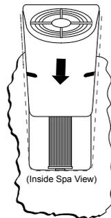
**J** Install filter cover by sliding it down into position over mating spa retainer clips. Turn spa power back on after skimmer cover is installed.
