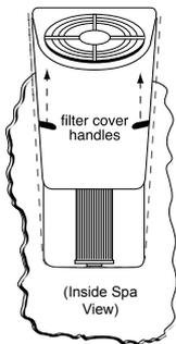
**B** Lift upward on filter skimmer cover handles to remove it from mating retainer clips.
