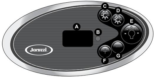
B. **Heat Indicator:** Lit when heater is on.
