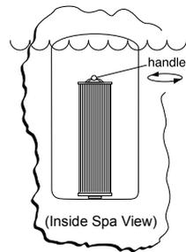
**D** Rotate filter cartridge handle counterclockwise to unthread filter cartridge from mating wall fitting.
