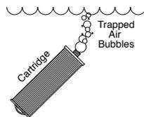
**G** Submerge filter cartridge in spa. Tilt threaded end upward to remove trapped air bubbles, then keep cartridge submerged to prevent air entrapment during installation (step H).
