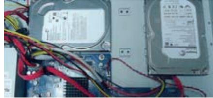
3) Turn over the machine and secure the HDDs with the screws and then install back the top cover.
