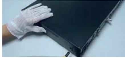
2) Put the HDD onto the bottom case and then connect the power and data cables.
