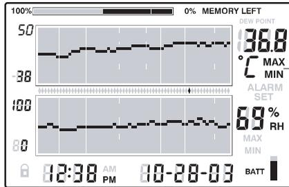
MAX or MIN indicator is ON when in the MAX or MIN mode
