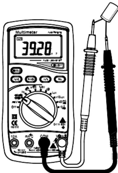
IN QUESTA MODALITÀ NON PUÒ ESSERCI NEL CIRCUITO DI MISURA ALCUNA TENSIONE. SCARICARE I CONDENSATORI.
